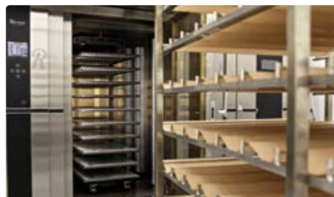
3. The Rotosole unit is stationed and pre-heated in the oven. All you need to do is enter the Rotosole racks with the soft trays and close the door.
