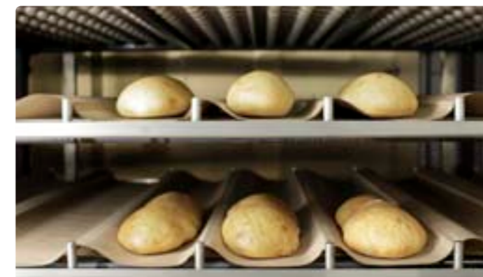
4. The Rotosole unit is elevated – bringing the bread in contact with its hot aluminum surface.
